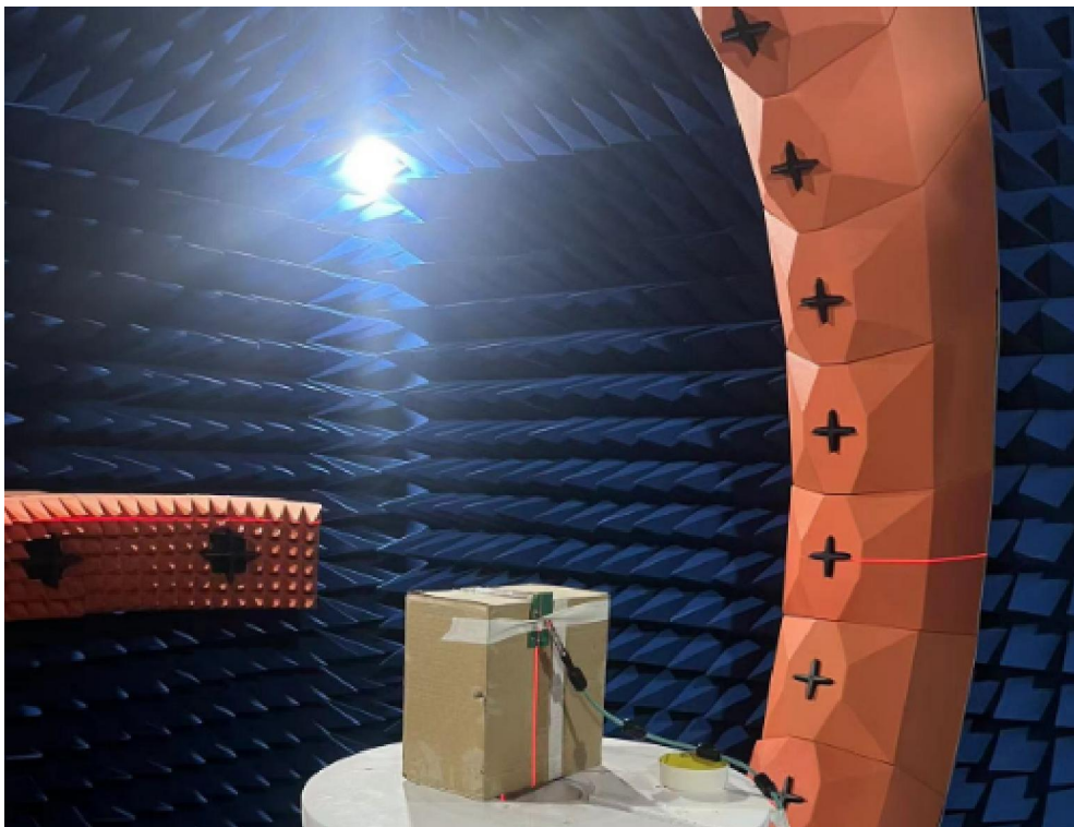
Figure 8. The Gain pattern is measured in FAR-field chamber
