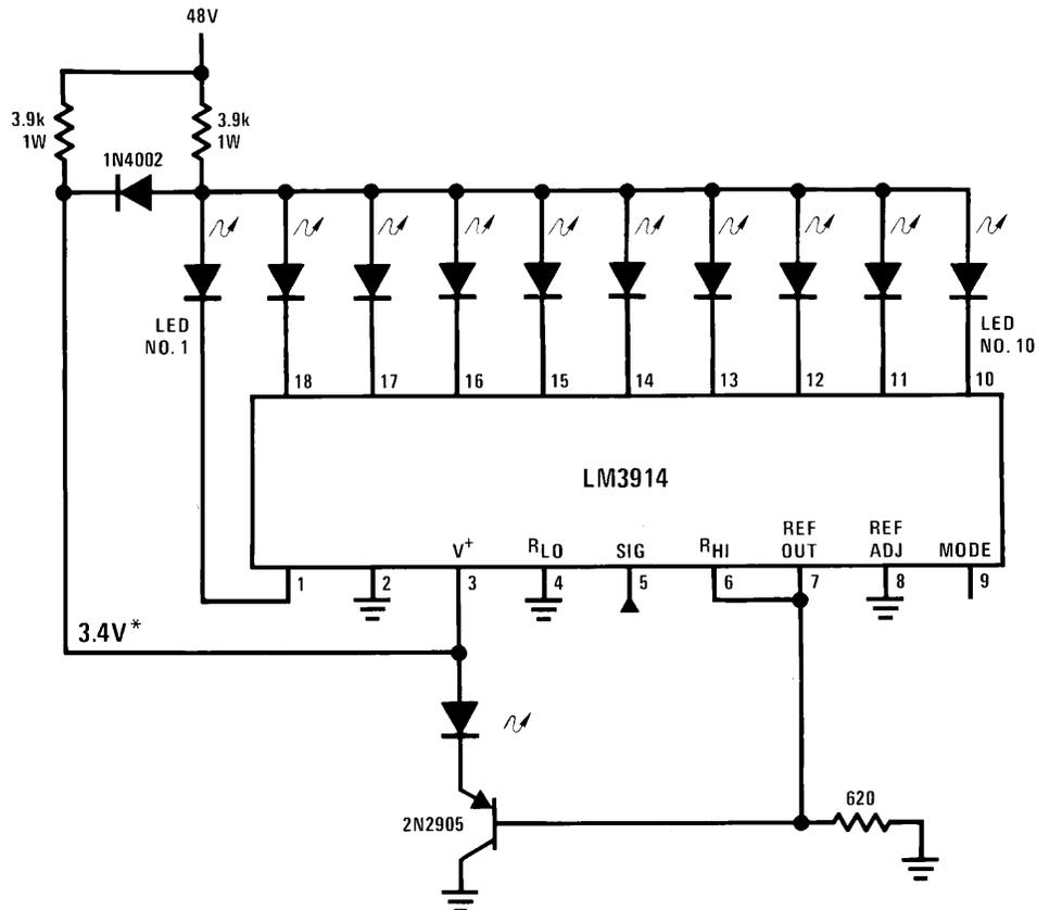
The LED currents are approximately 10mA, and the LM3914 outputs operate in saturation for minimum dissipation.
