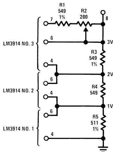
Figure 27. Adjusting Linearity of Several Stacked Dividers
