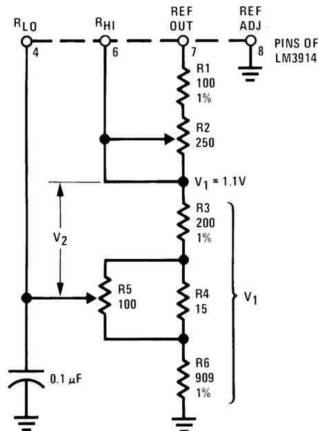
Figure 25. Greatly Expanded Scale (Bar Mode Only)
