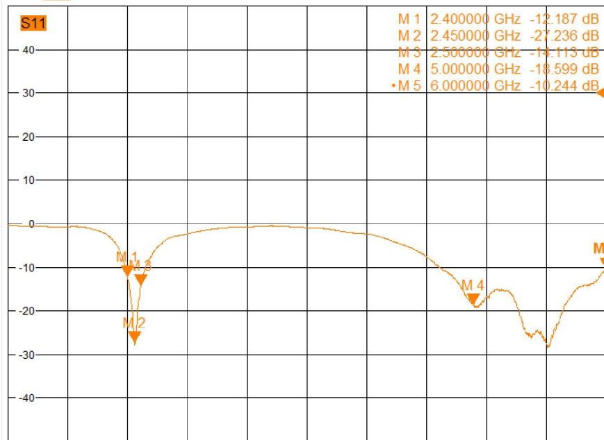
Figure 7. MAN2458C50 Return Loss
