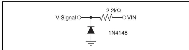
Figure 42. Enhanced Protection Against Negative Overload of  $V_{IN}$
