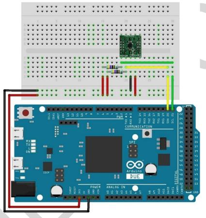
The EV3479A evaluation board can be easily wired to any microcontroller. This example shows a typical Arduino DUE platform. For other microcontrollers, be sure it has I2C with repeated-start support, then port the code. Please refer to the illustration below to connect the related pins.
