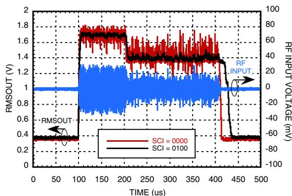
**Residual Ripple for 1.9 GHz WIMAX OFDM
