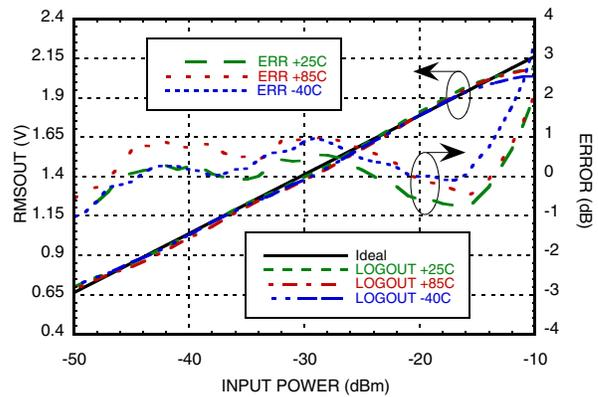
**RMSOUT & Error vs. Pin @ 2700 MHz [1][2]**
