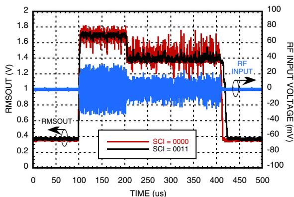
**Residual Ripple for 1.9 GHz WIMAX OFDM
