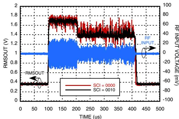
**Residual Ripple for 1.9 GHz WIMAX OFDM
