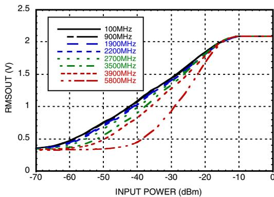
**RMSOUT Error vs. Pin with CW @ +25 °C [1]**
