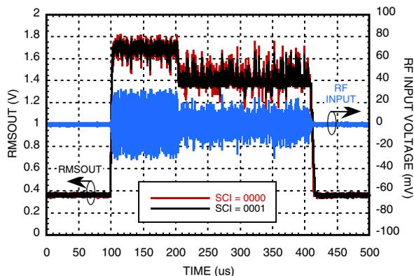
**Residual Ripple for 1.9 GHz WIMAX OFDM
