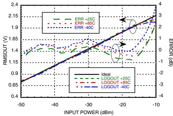
**RMSOUT & Error vs. Pin @ 900 MHz [1][2]**
