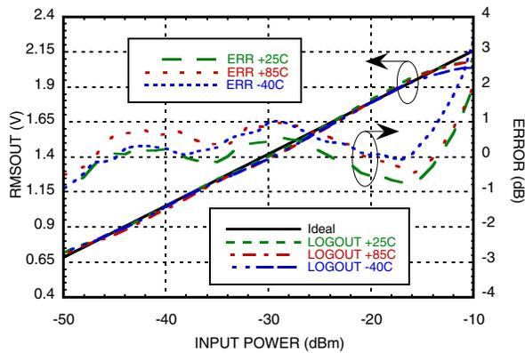
**RMSOUT & Error vs. Pin @ 2200 MHz [1][2]**
