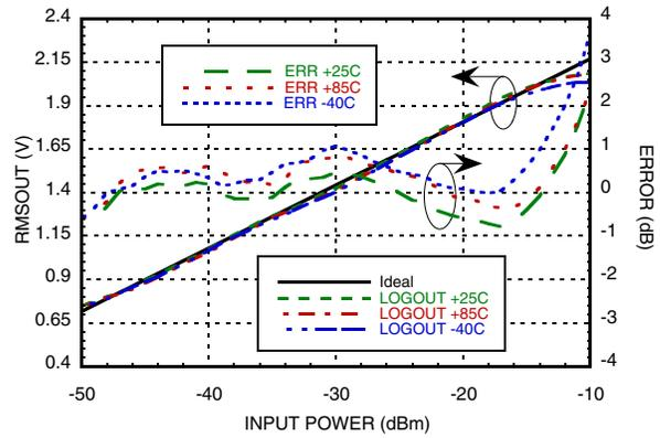
**RMSOUT & Error vs. Pin @ 1900 MHz [1][2]**
