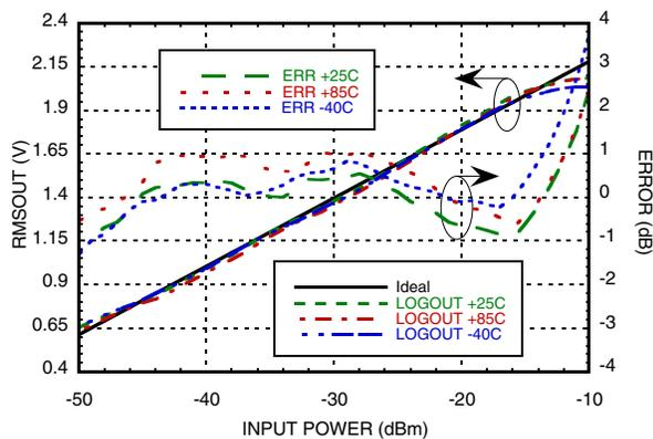
**RMSOUT & Error vs. Pin @ 3500 MHz [1][2]**
