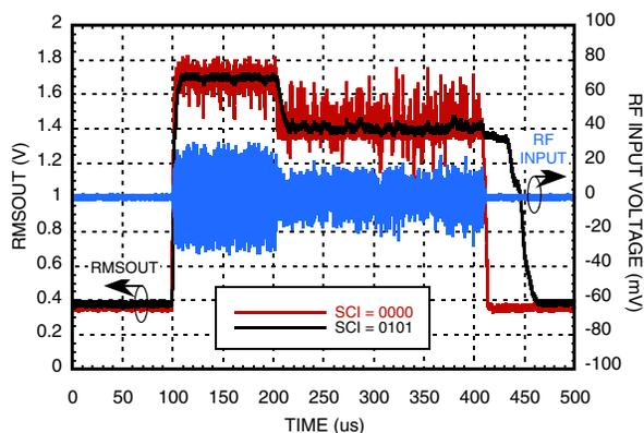
**Residual Ripple for 1.9 GHz WIMAX OFDM
