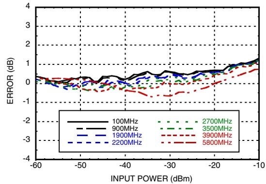
**RMSOUT vs. Pin with CW @ +25 °C [1]**
