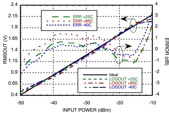
**RMSOUT & Error vs. Pin @ 5800 MHz [1][2]**
