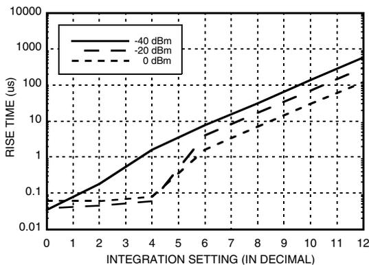
**Rise Settling Time<sup>[2]</sup> vs. SCI Setting over Input Power**
