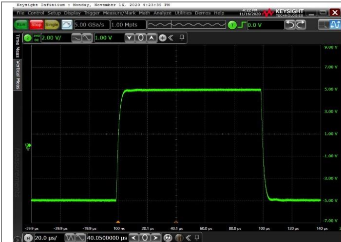
Voltage: 2V/div for Output, Time: 20us/div G=100, VREF = GND; VIN=0.1VPP, Load R=10K C=100pF
