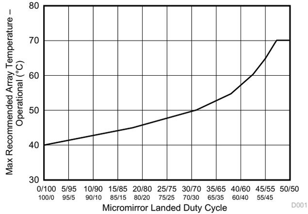
图 6-1. Maximum Recommended Array Temperature - Derating Curve
