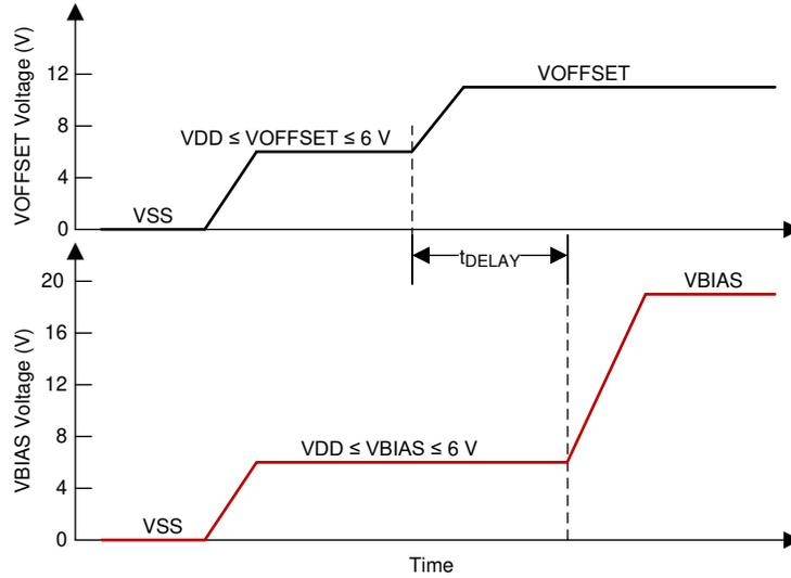
Refer to 表 9-1 for VOFFSET and VBIAS supply voltage levels during power-up sequence delay.
