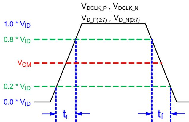
图 6-4. SubLVDS Input Rise and Fall Slew Rate
