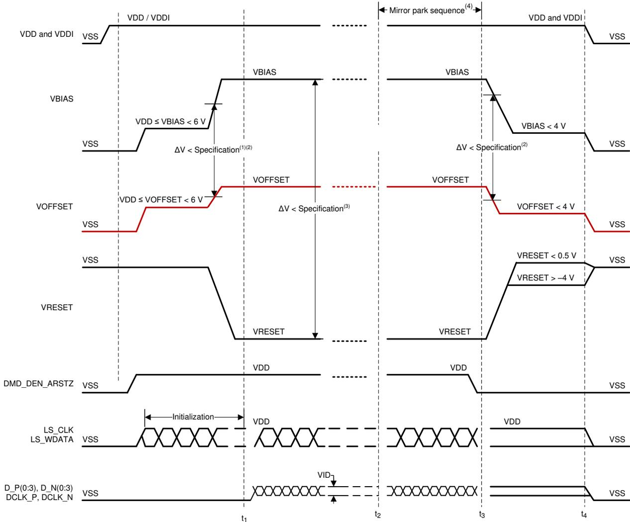
DLP controller and PMIC controls start of DMD operation
