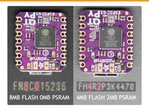
It can be tricky to tell which variant of the board you have. On the chip there is some text that denotes flash and ram size. If you see the text **FN8C0**, then it is the 8MB Flash/No PSRAM version. If you see the text **FH4R2**, then it is the 4MB Flash/2MB PSRAM version.
