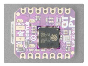
The ESP32-S3 is a highly-integrated, low-power, 2.4 GHz Wi-Fi System-on-Chip (SoC) solution that now has WiFi and BLE support, built-in native USB as well as some other interesting new technologies like Time of Flight distance measurements. With its state-of-the-art power and RF performance, this SoC is an ideal choice for a wide variety of application scenarios relating to the Internet of Things (IoT) (https://adafru.it/Bwq), wearable electronics (https://adafru.it/Osb), and smart homes.
