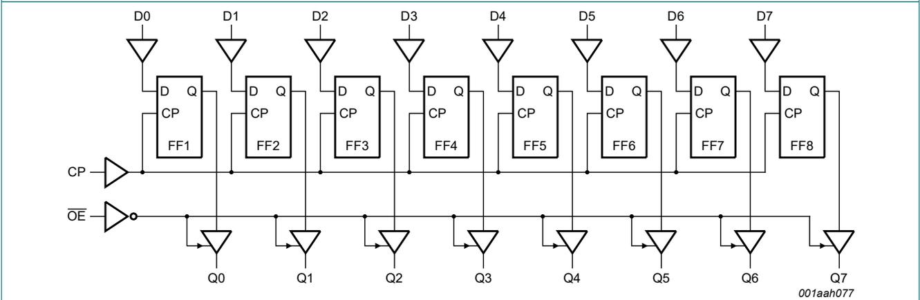
Fig. 2. Logic diagram
