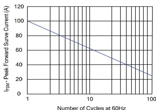
Figure 6 Maximum Non-Repetitive Forward Surge Current Uni-Directional Only
