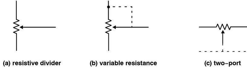
Figure 6. Potentiometer Configuration
