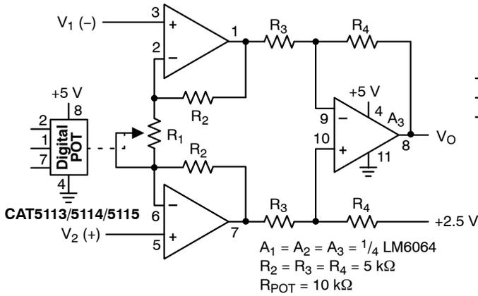
Figure 7. Programmable Instrumentation Amplifier
