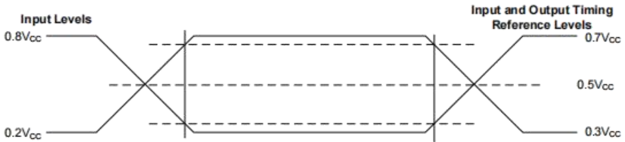
Figure 10.3 AC Measurement I/O Waveform
