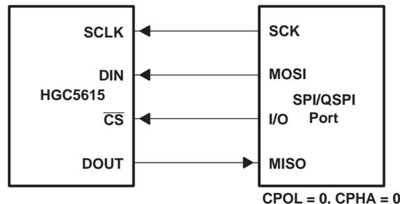
NOTE A: The DOUT-MISO connection is not required for writing to the HGC5615 but may be used for verifying data transfer.
