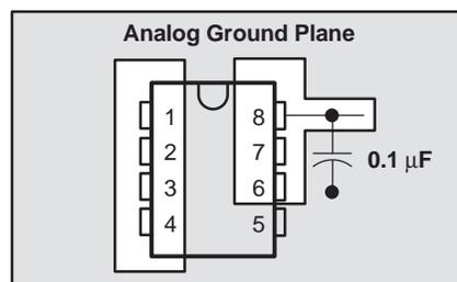
**Figure 15. Power-Supply Bypassing**
