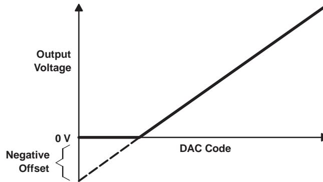
**Figure 14. Effect of Negative Offset (Single Supply)**
