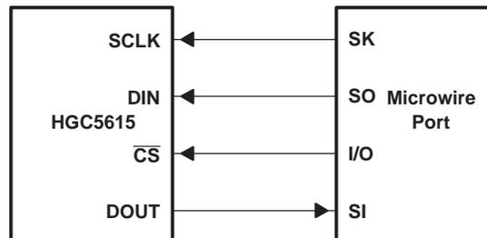
NOTE A: The DOUT-SI connection is not required for writing to the HGC5615 but may be used for verifying data transfer if desired.
