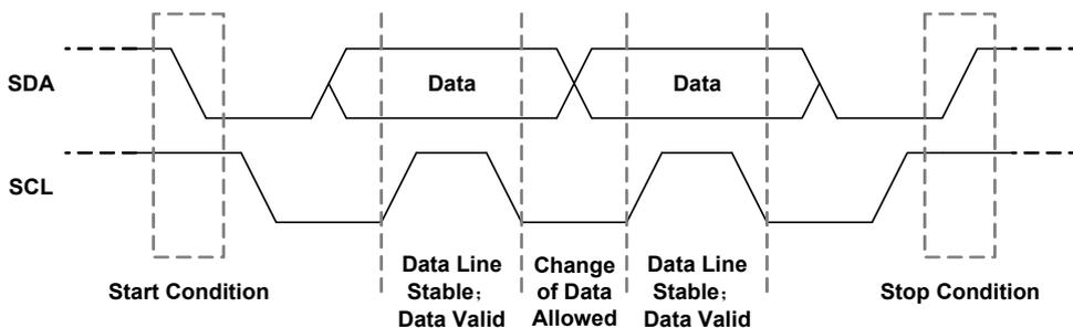
**Figure 2. Start Condition, Stop Condition, and Data Bit Transmission in I<sup>2</sup>C Communication**
