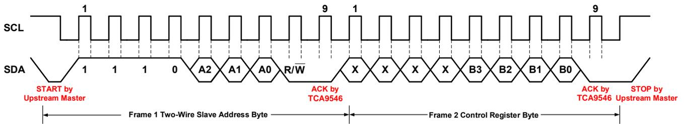
**Figure 3 Diagram of Control Register Write Operation**
