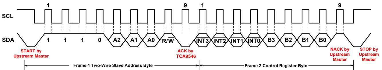
**Figure 4 Diagram of Control Register Read Operation**
