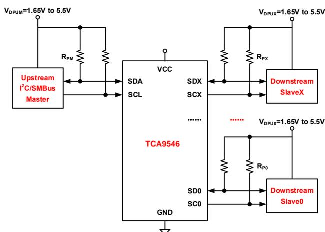
Figure 5 Diagram of Data Transmission Across Voltage Domains
