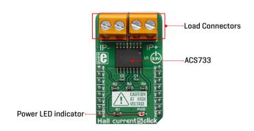
The ACS733 senses current differentially, allowing higher precision and good rejection ratio of common-mode interferences. The output voltage changes linearly with the current in the primary circuit, with the ratio of 66mV/A, and it is available at the AN pin of the mikroBUS™. Each IC is factory-calibrated, yielding a total output error as low as 1% while operated in the temperature range from 25°C to 125°C, measuring 20A through the primary conductor.
