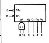
Vcc = Pin 14 GND = Pin 7 NC = Pins 1, 2, 3, 6
