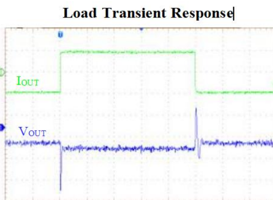
CH1: V_{OUT} (50mV/DIV) CH3: I_{OUT} (50mA/DIV) V_{IN}=10V , I_{OUT}=10mA-100mA 改变
