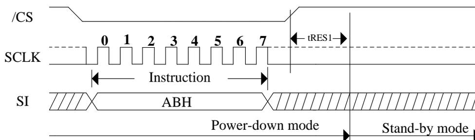
Figure 15b. Release Power-Down/Read Device ID Sequence Diagram
