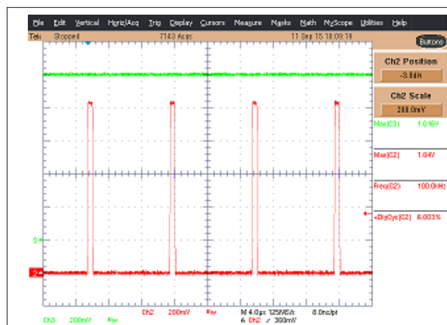
图 8-8. Supply Voltage 2.2 V, Peak Signal 1 V
