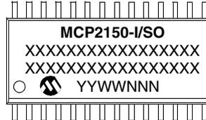
20-Lead SSOP (209 mil, 5.30 mm)
