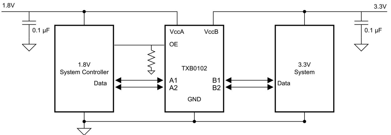
**Figure 7. Typical Operating Circuit**
