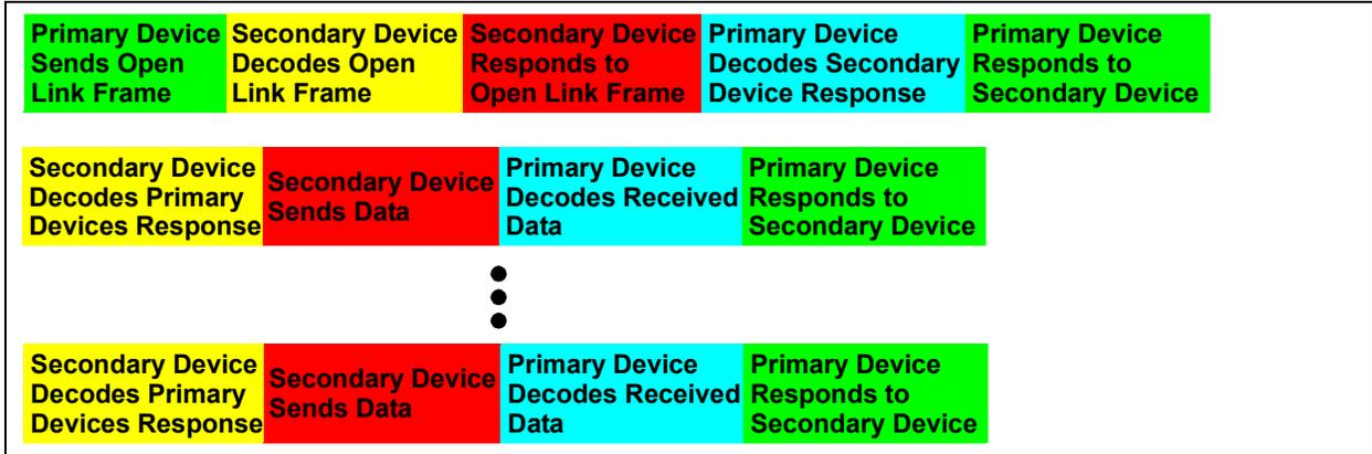
**FIGURE 2-12: HOST CONTROLLER TRANSMISSION (S → P) OF A 250 BYTE PACKET (TO PIC IrDA STANDARD STACK)**
