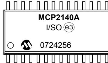
20-Lead SSOP (209 mil, 5.30 mm)
