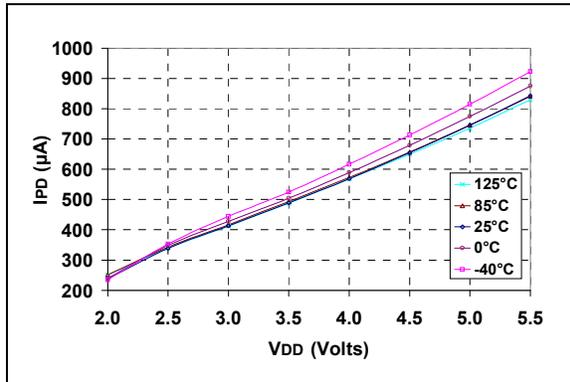
**FIGURE 5-2: IDD (PHACT = L) VS. TEMPERATURE**
