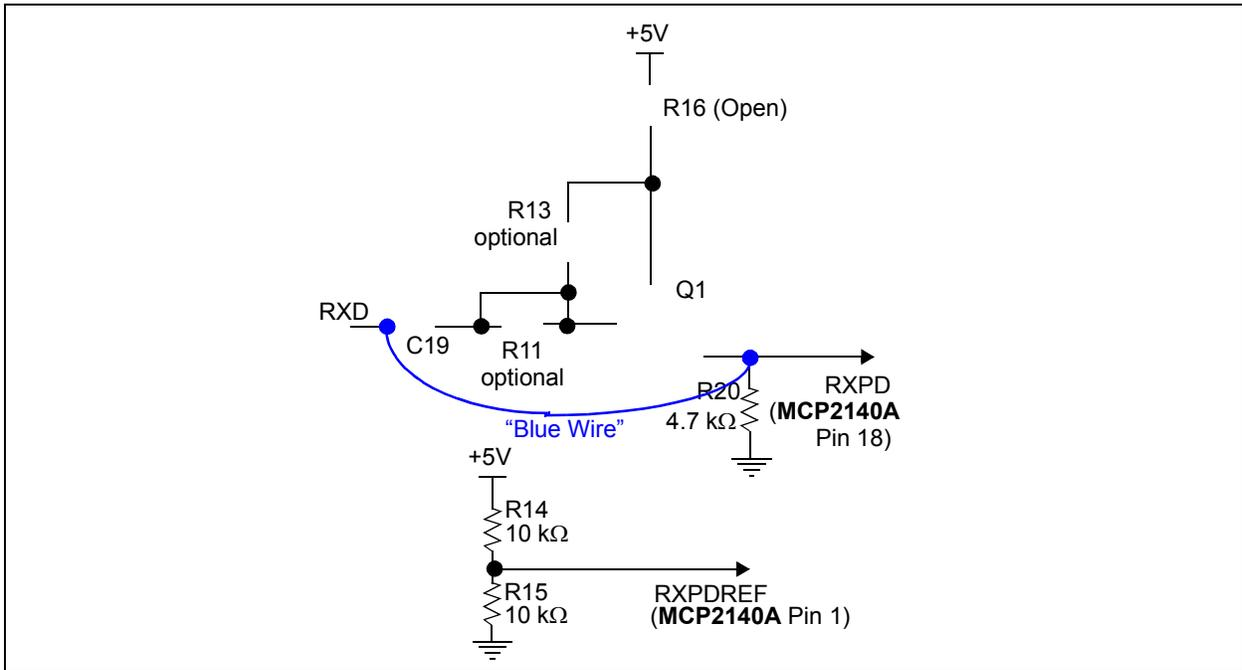
**FIGURE 2-19: MCP2140A MODIFICATIONS OF MCP2140 WAVE SHAPING CIRCUIT**
