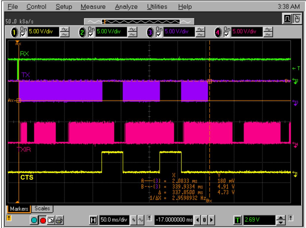
FIGURE 2-5: HOST UART CTS FLOW CONTROL FLOWCHART
