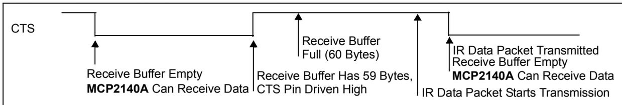
**FIGURE 2-11: EXAMPLE IR COMMUNICATION SEQUENCE**
