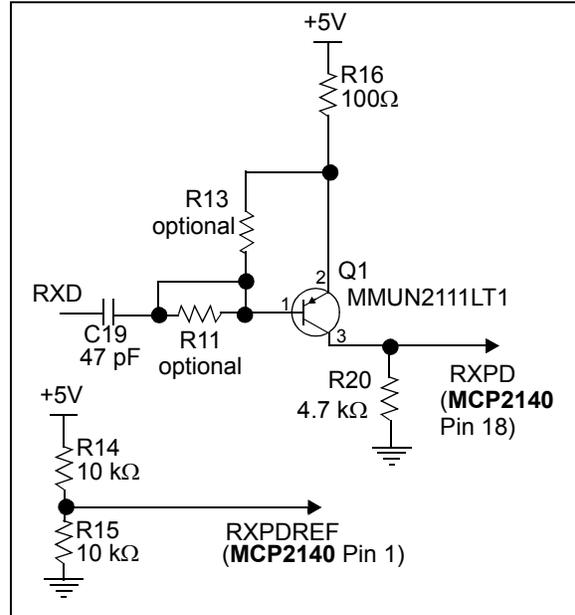
**FIGURE 2-17: MCP2140A MODIFICATIONS OF MCP2140 WAVE SHAPING CIRCUIT**
