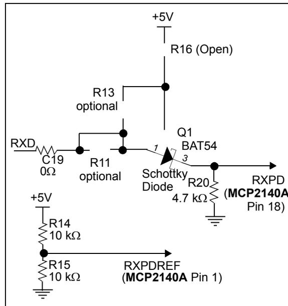
**FIGURE 2-18: MCP2140A “BLUE WIRE” MODIFICATIONS OF MCP2140 WAVE SHAPING CIRCUIT**
