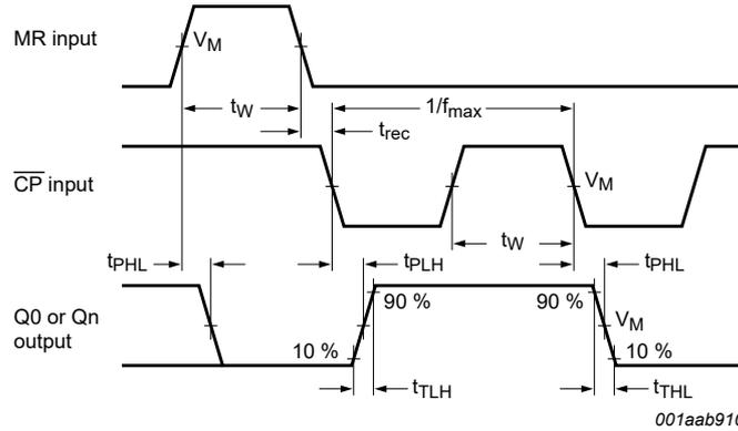
Also showing the master reset (MR) pulse width, the master reset to output (Qn) propagation delays and the master reset to clock (CP) recovery time.
