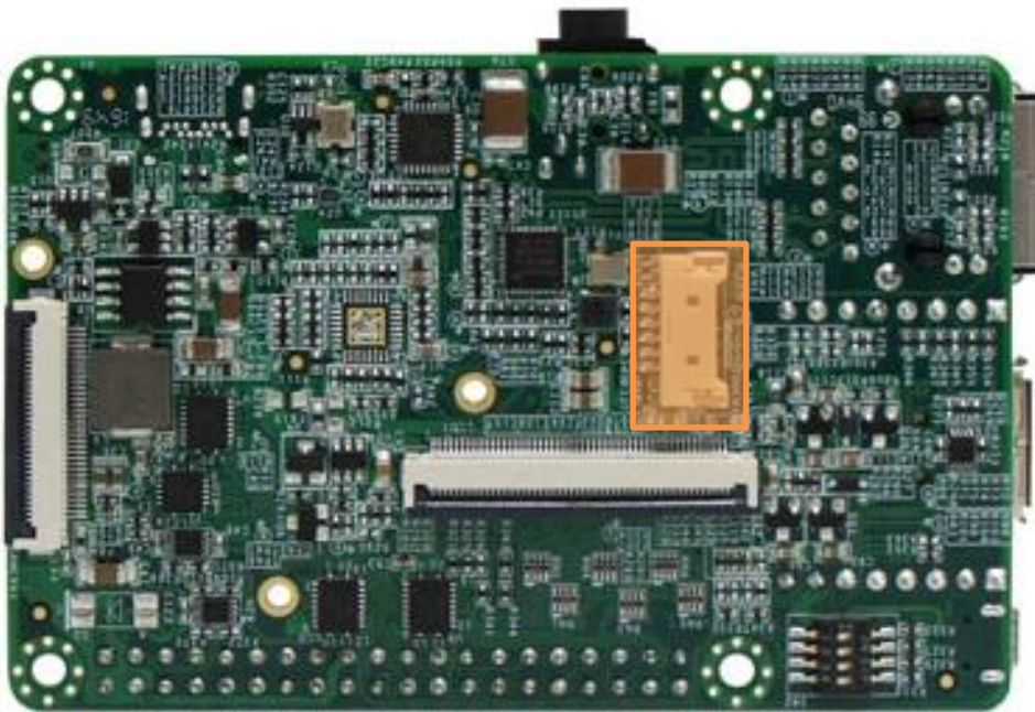
Figure 22 - PICO-PI-IMX6UL Touch Panel Connector Location
