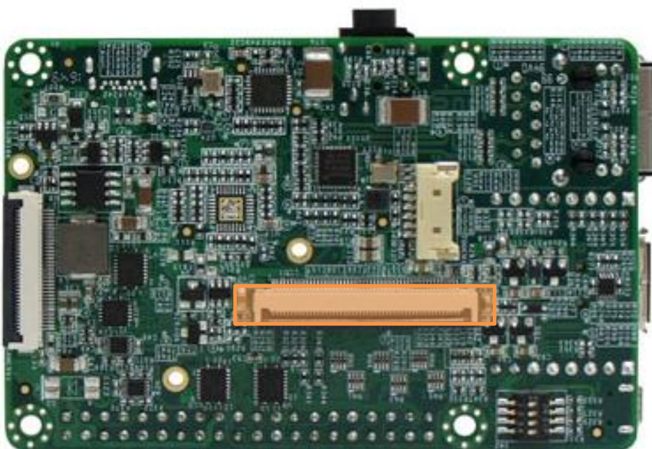
Figure 21 - PICO-PI-IMX6UL LCD Display FPC Connector Location
