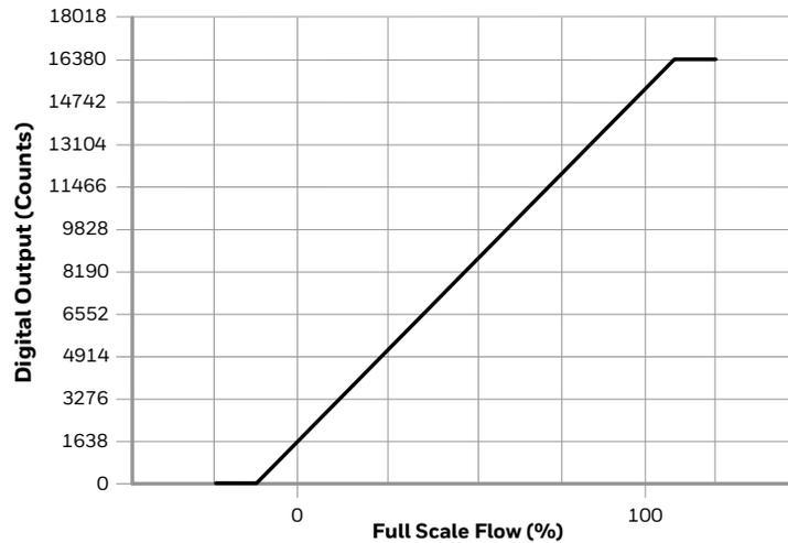
Figure 5. Accuracy and Total Error Band
