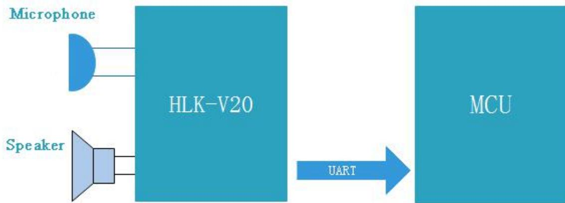
Figure 6 Module application example diagram
