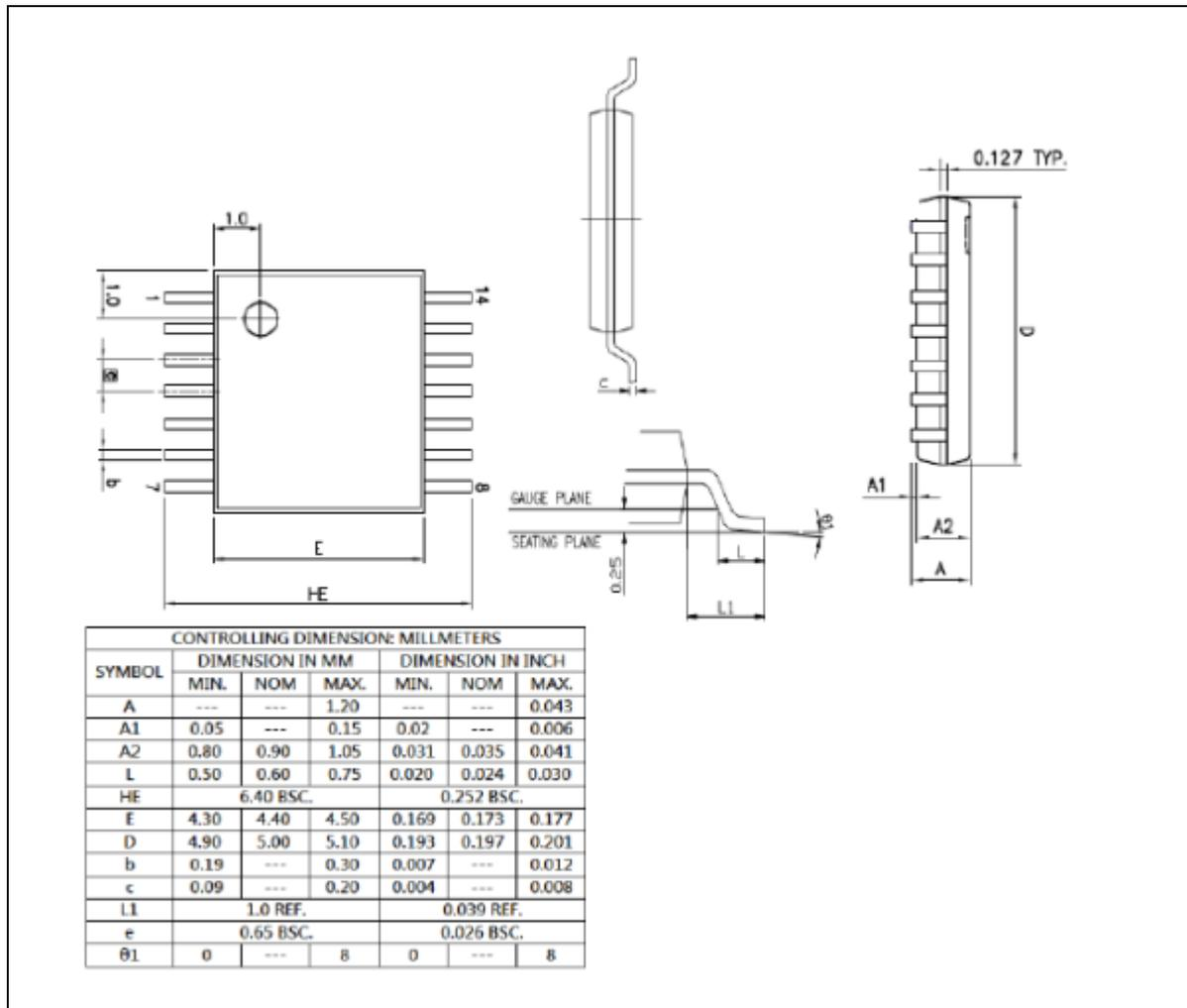
7.8 MSOP 10 (3x3 mm) for MS51BA9AE
