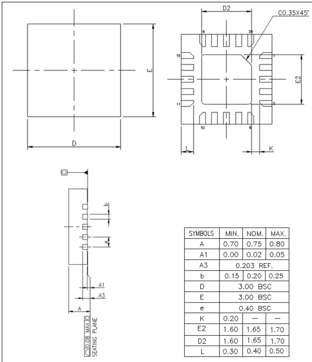
7.6 QFN 20 (3.0x3.0 mm) for MS51XB9BE & MS51XC0BE
