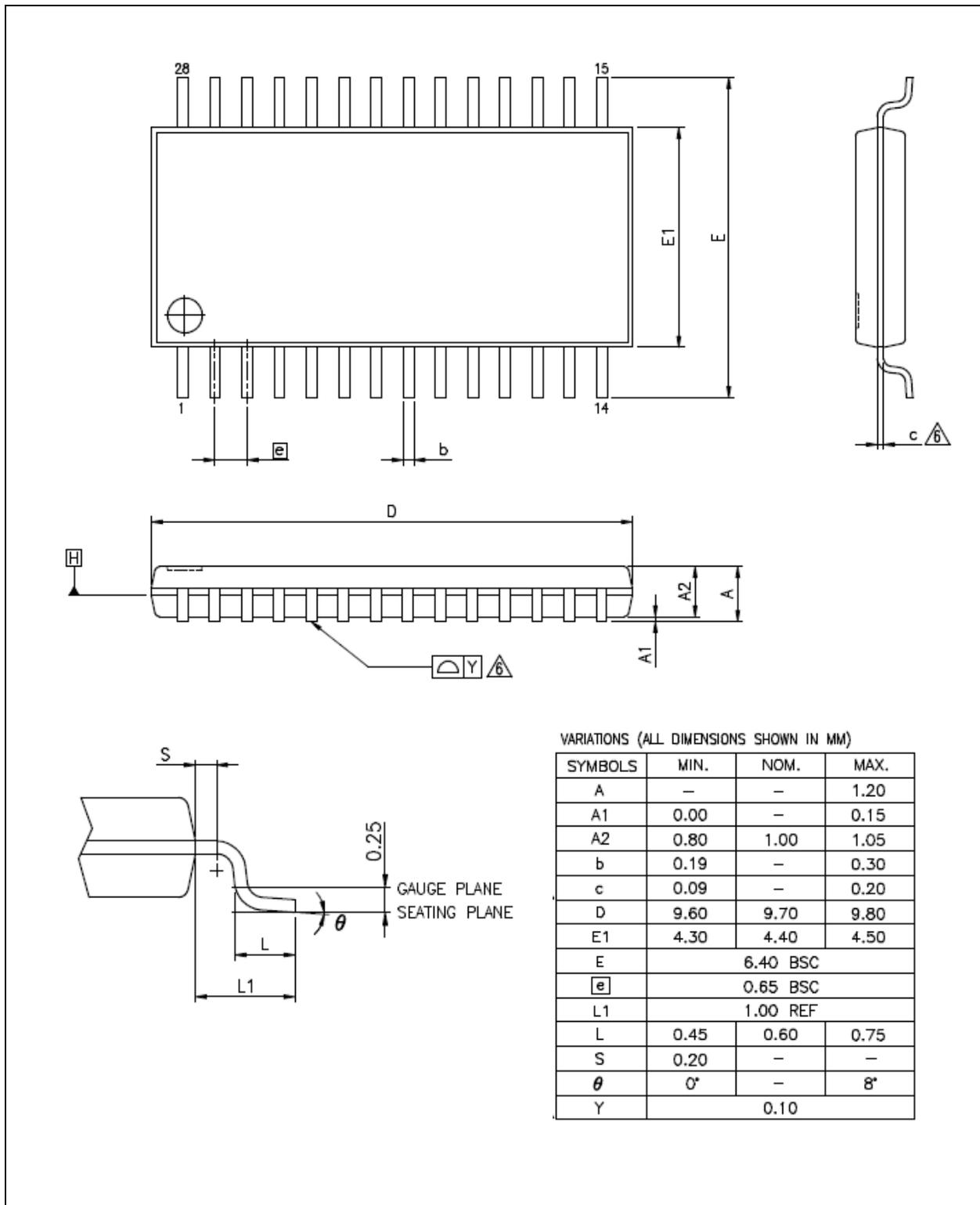
7.4 TSSOP 20-Pin (4.4x6.5x0.9 mm) for MS51FB9AE & MS51FC0AE
