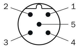
Connector M12, 5-pin, A-coded
