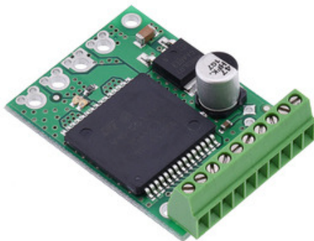
0.1" screw terminal block being used with a VNH5019 motor driver carrier in place of the included 0.1"-pitch male header.
