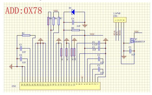
The I2C communication interface consists of slave address bit DC, I2C-bus data signal SDA (SDAOUT/D2 for output and SDAIN/D1 for input) and I2C-bus clock signal SCL (D0). Both the data and clock signals must be connected to pull-up resistors.
