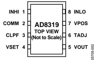
Figure 2. Pin Configuration
