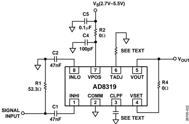
Figure 22. Basic Connections
