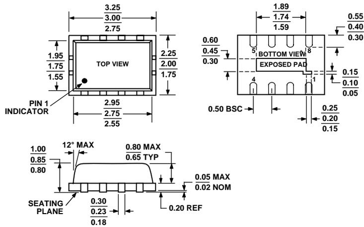
Figure 39: 8-Lead Lead Frame Chip Scale Package [LFCSP\_VD]
