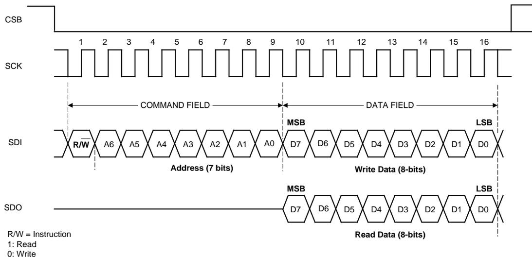
Figure 12. SPI Transaction Format
