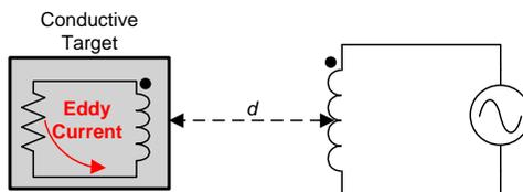
Figure 46. Conductor in an AC Magnetic Field
