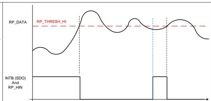
**Figure 57. INTB/SDO Output for R<sub>P</sub> Threshold High (INTB\_FUNC=b00'00011)**
