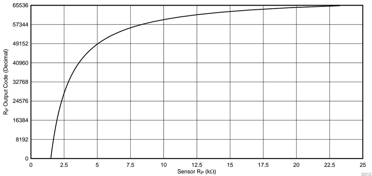
**Figure 50. LDC1101 R<sub>p</sub> Transfer Curve with R<sub>P</sub>MIN = 1.5 kΩ and R<sub>P</sub>MAX = 24 kΩ**
