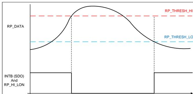
**Figure 56. INTB/SDO Output Value for R<sub>P</sub> Comparator with Hysteresis (INTB\_FUNC=b00'0010)**
