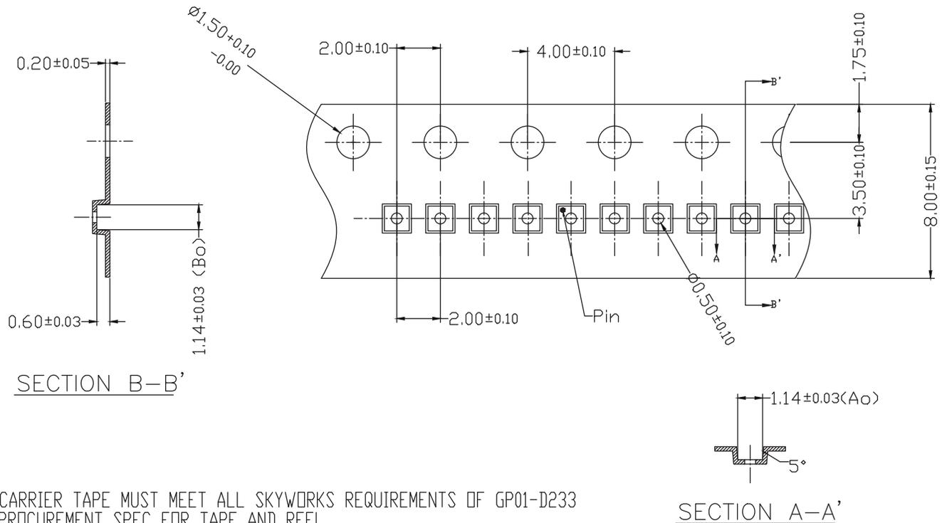
1. CARRIER TAPE MUST MEET ALL SKYWORKS REQUIREMENTS OF GP01-D233 PROCUREMENT SPEC FOR TAPE AND REEL
