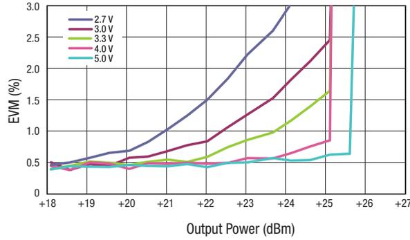
Figure 9. 802.11a EVM vs Output Power, 5.2-5.8 GHz, 54 Mbps
