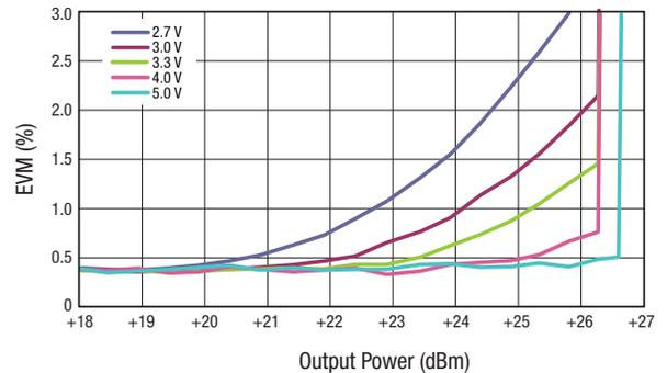
Figure 8. 802.11g EVM vs Output Power @ 2.45 GHz, 54 Mbps
