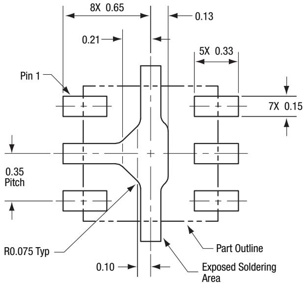
All measurements in millimeters
