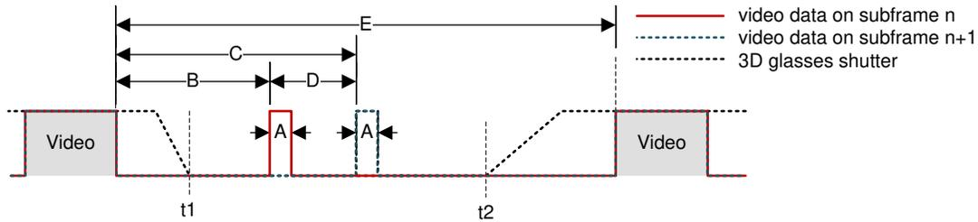
The time offset of DLP Link pulses at the end of a subframe alternates between B and B+D where D is the delta offset.
