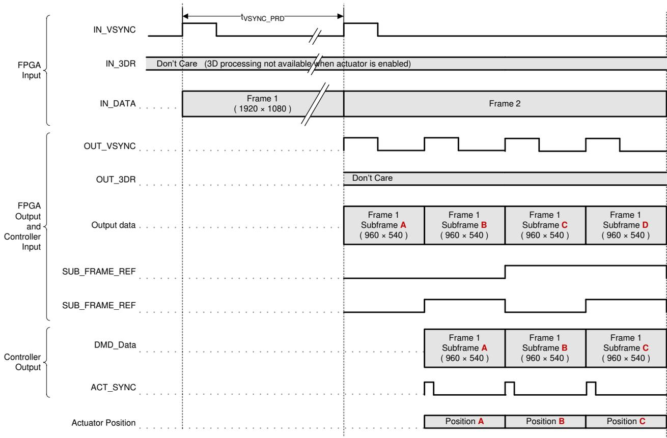
图 7-1. 2D Actuator Frame and Signal Timing
