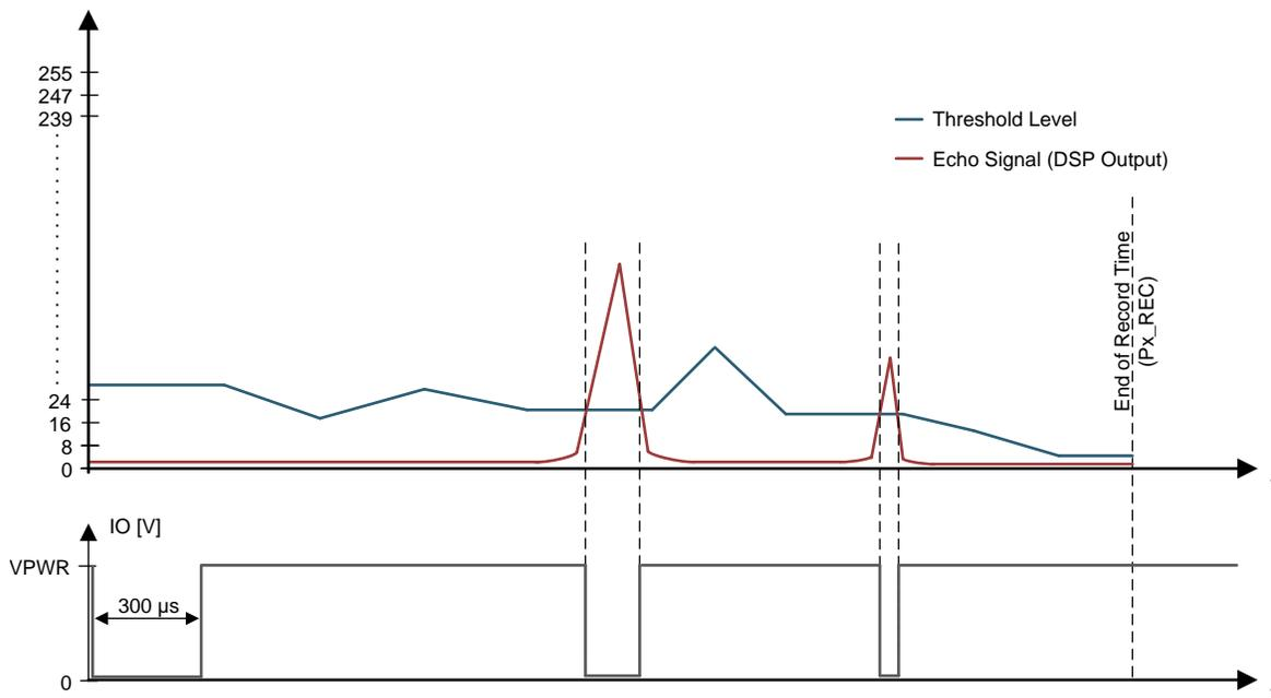
图 16. IO-Pin Object-Detection Signaling With Listen-Only Time Command
