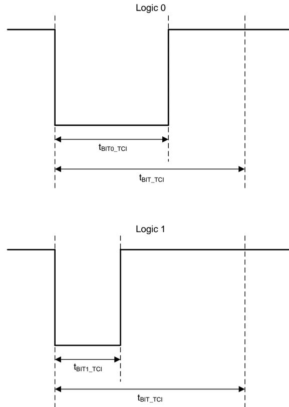
**图 13. Time-Command Interface Bit Timing**
