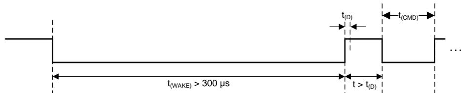
图 37. Time Command Interface Wake-Up Pulse
