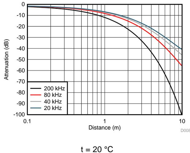
图 137. Attenuation Characteristics of Sound Pressure by Distance
