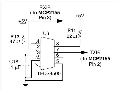
The optical transceiver logic can be implemented with discrete components, for component cost savings. Care must be taken in the design and layout of the photo detect circuit. This is due to the small signals that are being detected and their sensitivity to noise. A discrete implementation of the optical transceiver logic is implemented on the MCP2120 and MCP2150 Developer's Kit boards.
