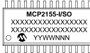
20-Lead SSOP (209 mil, 5.30 mm)
