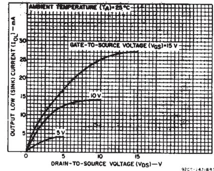
Fig. 3 – Typical n-channel output low (sink) current characteristics.
