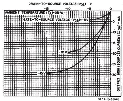
Fig. 5 - Typical p-channel output high (source) current characteristics.
