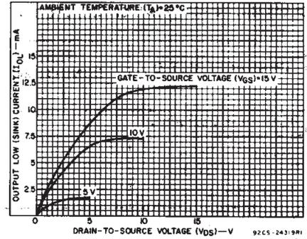
Fig. 4 - Minimum n-channel output low (sink) current characteristics.
