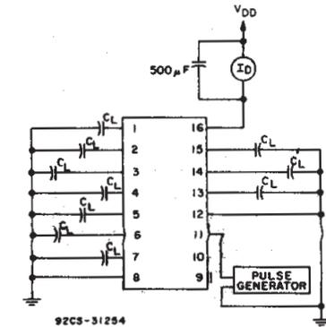
Fig. 11 - Dynamic power dissipation test circuit.
