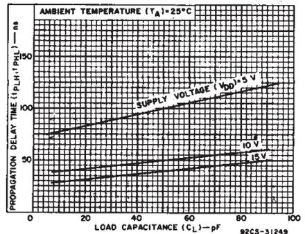
Fig. 7 - Typical propagation delay time (Q<sub>n</sub> to Q<sub>n+1</sub>) as a function of load capacitance.
