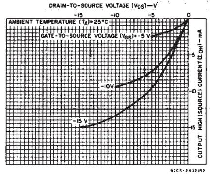
Fig. 6 - Minimum p-channel output high (source) current characteristics.
