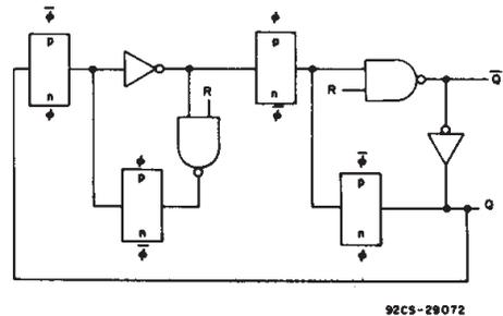
Fig. 2 – Detail of typical flip-flop stage.
